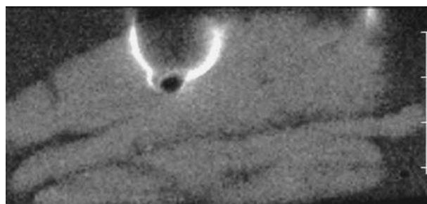
Fig. 5. MRI artifacts caused by the Neurovent-P® ICP probe implanted in a fresh pig brain specimen imaged at 1.5 Tesla using a T1-weighted spin-echo sequence
